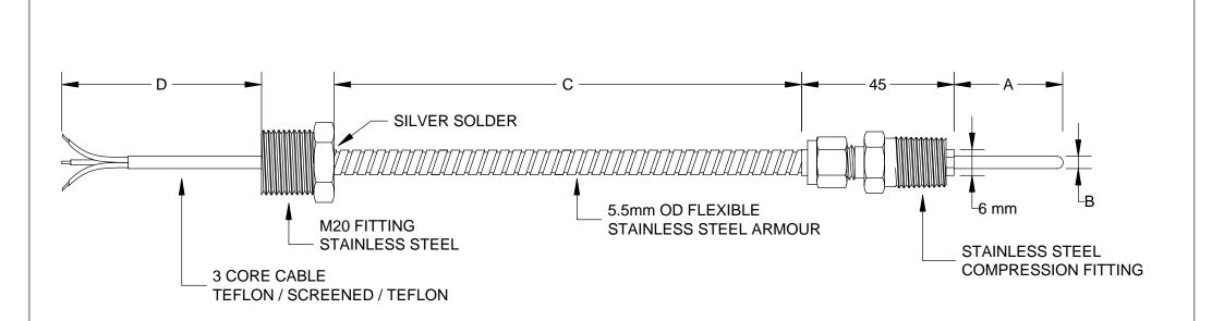
RTD PT100 SENSOR 3 WIRE ALL STAINLESS STEEL COMPONENTS ARMOUR COVERED LEADS
